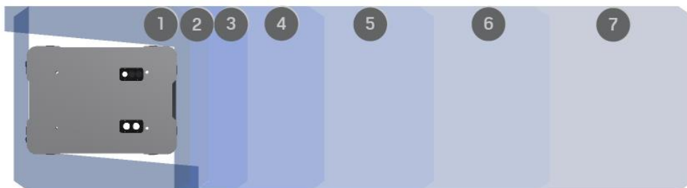
Figure 2.14. The illustration shows the field set contours when driving forward. The range of the field set changes with the robot's speed.
